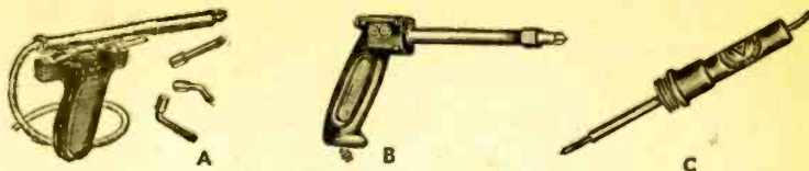
Fig. A—75 AND 125 WATT "GUN GRIP" SOLDERING IRONS
